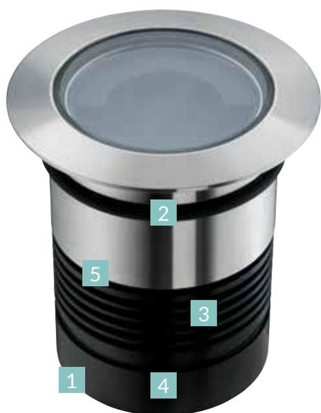
1. The Smart Shield protects against polarity inversion; an integrated super fast diode prevents accidental damage to the luminaire during installation due to reverse polarity.
